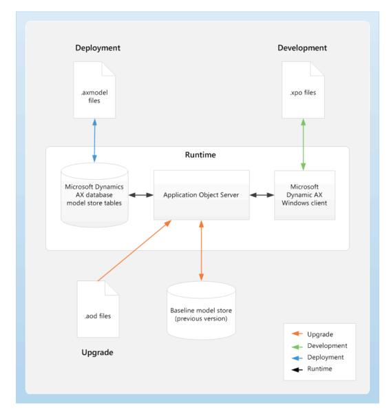
The following diagram provides an overview of the model store architecture.
