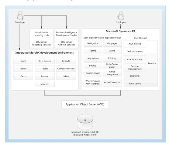
The following figure illustrates the high-level client architecture.
