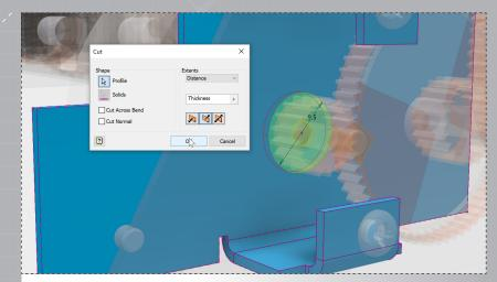
Click the green check in the ribbon to finish the sketch. Select 'Cut' from the marking menu and pick both circles in the sketch as the 'Profile' and select 'OK'.
