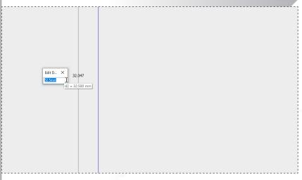
Right click and select 'General Dimension'. Select the left vertical line segment and click to place the dimension. Type in 32.5mm and touch 'Enter' on your keyboard to finish.
