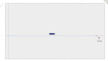
Click the origin point to start the line and then move your cursor to the right. Before you click the end point, type 62.5mm into the dynamic dimensioning box.
