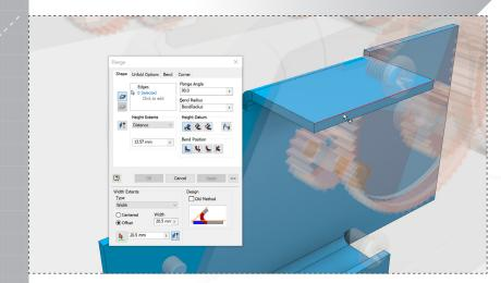
Select 'Apply' in the dialog to create the flange. Then select the edge as shown (flip if necessary).
