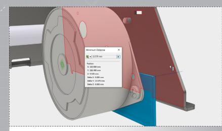
Right click and select 'Measure' from the marking menu. To determine the length of the flanges, measure from the outside edge of the bracket to inside edge of the part as shown.
