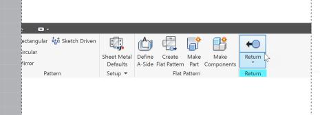
Hit 'OK' to complete the flange. Then select 'Return' in the ribbon menu to exit the editing environment and reactivate the entire assembly.
