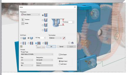
Restart the 'Hole' command from the ribbon. Select the centerpoints of the two circles in the sketch. Set the hole settings as shown. Click 'OK' to create the threaded holes. 10.
