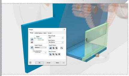
Use the 'Flip Direction' button in the dialog (if necessary) to make sure the new flange is in the correct orientation.
