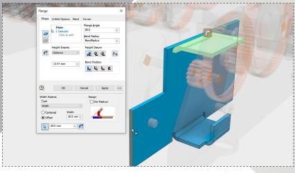
Again use 13.57mm for the 'Height Extents' and change the 'Width Extents' as shown. Click the arrow to select the face of the bracket as shown for the offset (flip if necessary).
