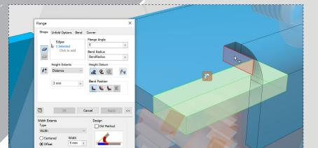
Change the 'Flange Angle' to O and configure the 'Height Extents' and 'Width Extents' as shown. Select the red highlighted face for the offset reference (flip if necessary).
