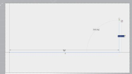
Click to set the end point of the line then move your cursor up. Type 18.5mm into the dynamic dimensioning box. Click to create the vertical line.
