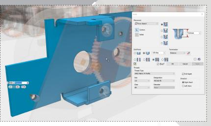
Restart the 'Hole' command from the ribbon. Select the centerpoints of the two circles in the sketch. Use the same threaded hole settings as before. Click 'OK' to create the threaded holes.
