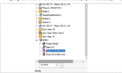
In the model browser, click to edit the 'Flush:27 (0.500 mm)' constraint to be -0.100 mm so the locator flange is aligned correctly in the assembly.
