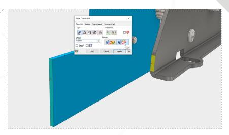
Select the two faces of the parts as shown. Type 0.5mm as the offset distance and in the 'Solution' section of the dialog select 'Flush'. Hit 'Apply' to create the constraint.
