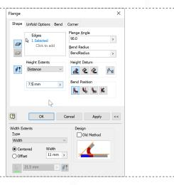
Configure the flange using the values and options for the 'Height Extents' and 'Width Extents' as shown. Click 'Apply' to create the flange.
