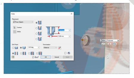
Pick the center point of the circle in the sketch and change the hole diameter in the dialog to 3.98mm. Select 'OK' to create the hole.
