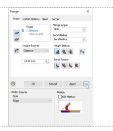
Enter the measured distance, 13.57mm, in the 'Height Extents' field and then expand the dialog by clicking the double arrows next to the 'Apply' button.
