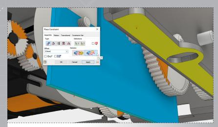
Rotate the model to view the bottom edge of the part. Select the two faces shown and use enter 3.5mm for the offset, continuing to use the 'Flush' constraint. Hit 'OK'.
