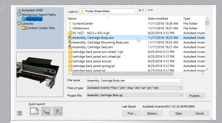
In Inventor, click the 'Projects' icon in the ribbon. Navigate to where you saved the files and select *Assembly, Cartridge Body. ipj*. Then open the file *Assembly, Cartridge Body.iam*.
