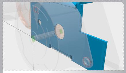
Rotate the model to view the back of the bracket. Start the 'Project Geometry' command and select the two circular features highlighted. Right click and select 'Finish 2D Sketch'.
