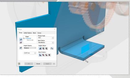
Click 'Apply' on the dialog to create the first flange. To start the second flange, select the edge as shown.
