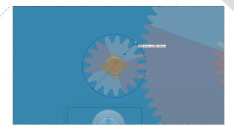
Start the 'Center Point Circle' from the marking menu. Select the center point of the projected geometry and enter 9.5mm in the dynamic dimension box and hit 'Enter'. Right click and 'OK'.
