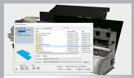
Inside the **Assembly, Cartridge Body.iam** assembly, right click and select 'Place Component'. Select the **SMB.ipt** file you just saved and select 'Open'.
