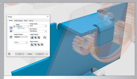
For the final flange, restart the 'Flange' command from the marking menu and select the edge as shown.
