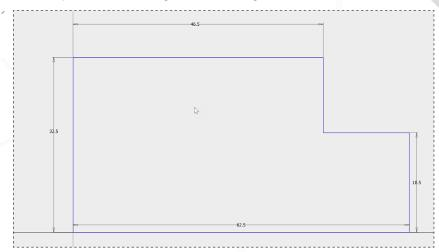
Repeat the process to add a 46.5mm dimension to the top horizontal line segment. The sketch is now fully constrained so click the green check mark in the ribbon to 'Finish Sketch'. 13
