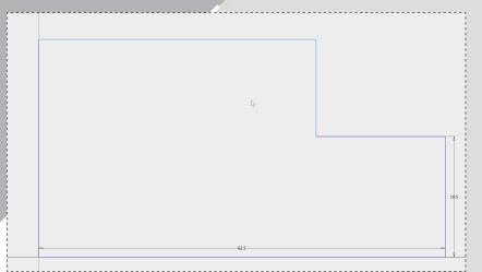
Continue to draw lines (without adding dimensions) to create the rough shape as shown. Ending on the origin point will complete the line segment, then right click and select 'OK'.
