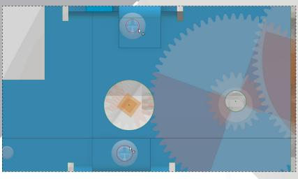
Start the 'Project Geometry' command from the marking menu. Select the two circular features highlighted above. Right click and select 'Finish 2D Sketch'.
