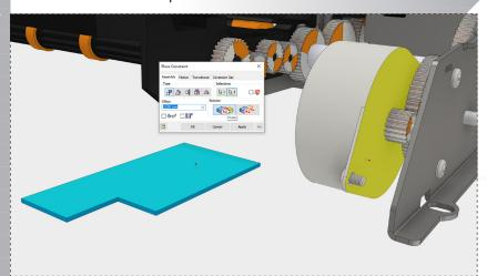
Right click and select 'Constraint' from the marking menu. Select the top face of the bracket and the inside face of the motor as shown. Hit 'Apply' to create the first constraint. 18.
