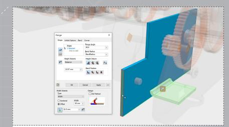
Change the 'Width Extents' type to 'Width' and enter 18mm. Select the 'Offset' button, enter 21.5mm in the field, and then click the arrow to select the face of the part as shown.
