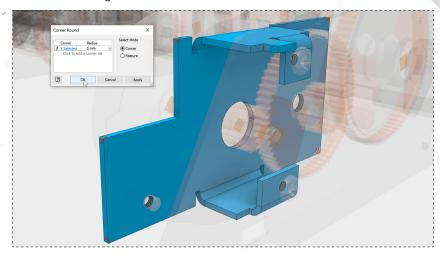
Select the edges as shown above and change the radius to 1mm. Click 'OK'. In the ribbon, select 'Return' to finish editing and save and close the files.
