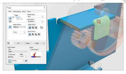
Configure the flange using the values and options for the 'Height Extents' and 'Width Extents' as shown. Select the face shown for the offset reference. Click 'OK'.
